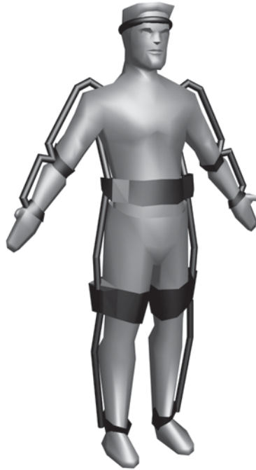
FIGURE 5.7 A mechanical Mocap system.
